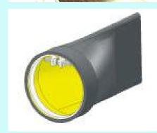
The Rhinoflex Series RFIN-E- Inline / expander type Duckbill check valve is a one way non return valve that are designed and engineered with a soft cuff that suits the Inside Diameter of the pipe. This consists of a round internal clamp, that when tightened, it clamps outward, onto the wall in the pipe. This enables the valve to be mounted on the inside of a pipeline, if there is no other way to secure the valve.
