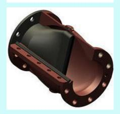
The Rhinoflex Series RFIN- J (Jacketed) INLINE Duckbill check valve is a one way non return valve that are designed and engineered for higher pressures, with a built-in flange that are part of the one piece elastomeric valve. This model is suitable when there is a requirement that prevents backflow, inside a pipe line. Suitable for higher line and back pressures.
