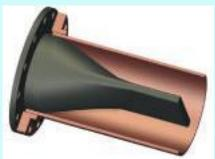
The Rhinoflex Series RFIN-INLINE Duckbill check valve is a one way non return valve that are designed and engineered with a built-in flange that are part of the one piece elastomeric valve. This model is suitable when there is a requirement that prevents backflow, inside a pipe line.
